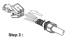
Put wires through wiring management in accordance with wiring color code.
