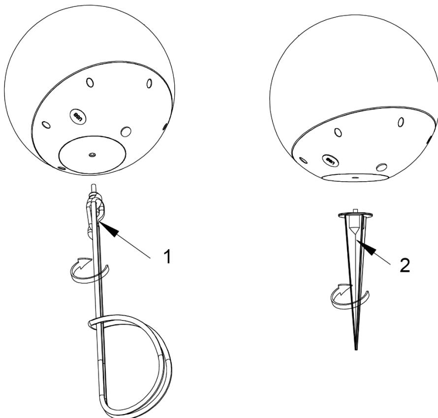
Use the hanging loop (1) to hang the lamp. Use the ground pin (2) to secure the lamp to the ground in your garden.
