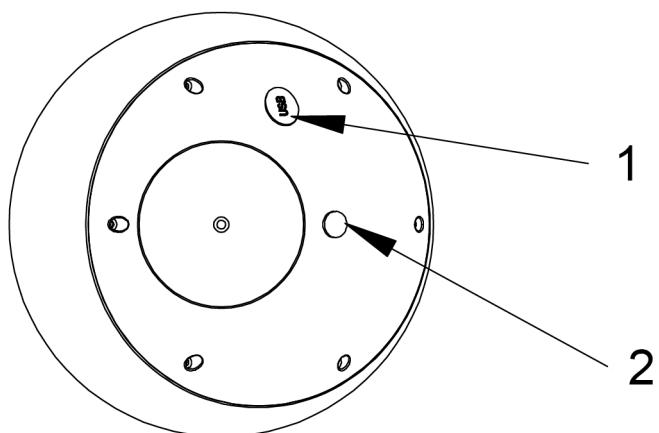
Connect the included USB cable to a computer or 5V adapter. Plug the MicroUSB end of the cable into the USB port of the lamp(1). After 3 hours, the lamp will be fully charged.
